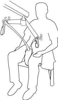
Feed the right leg support through the strap on the left leg support. Cross over leg straps, pass one leg strap through the other and attach to hoist on front hooks.
