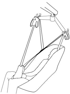
Raise lift to convenient height and attach the shoulder straps as shown. You may then raise the client to the required height. When seating the client the hand grip on the back of the sling may be used to ensure a good seated posture.
